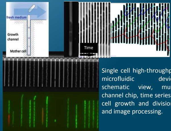
Single cell high-throughput microfluidic device: schematic view, multi-channel chip, time series of cell growth and divisions, and image processing.
